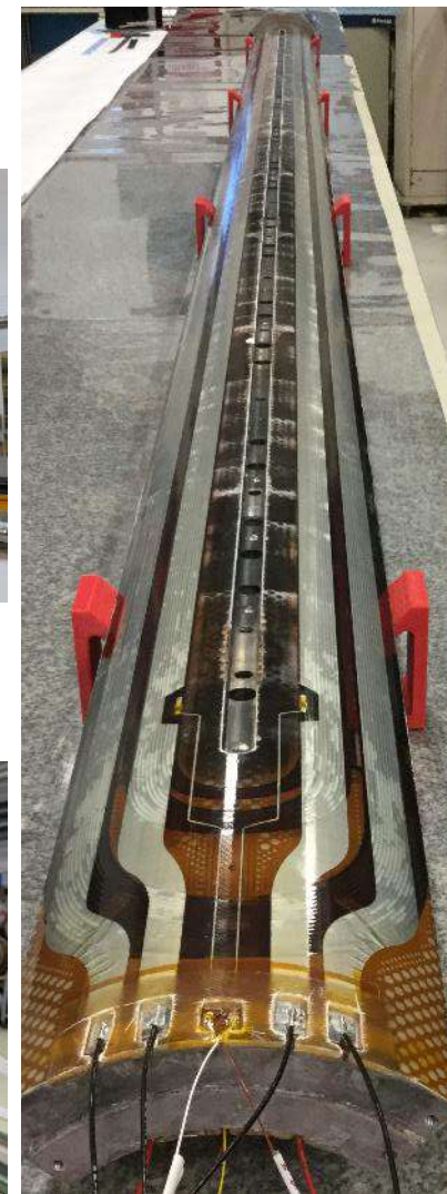
IR quad. Construction of the first 7.2 m magnet started at CERN
