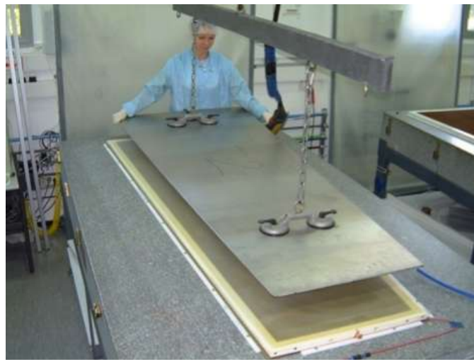
Figure 7.8: 1/2 chamber after being released from the winding machine with the wires already soldered.
