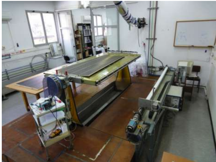
Figure 7.8: 1/2 chamber after being released from the winding machine with the wires already soldered.
