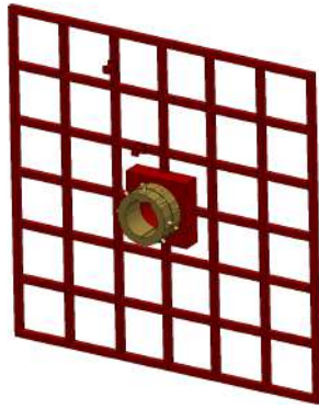
(a) The hub and the spoke mounts are attached to the support grid.
