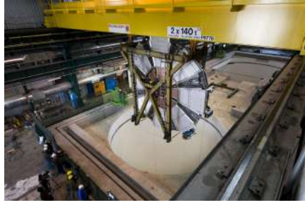
(a) A SW being picked up by the overhead crane at the surface in SX1.
