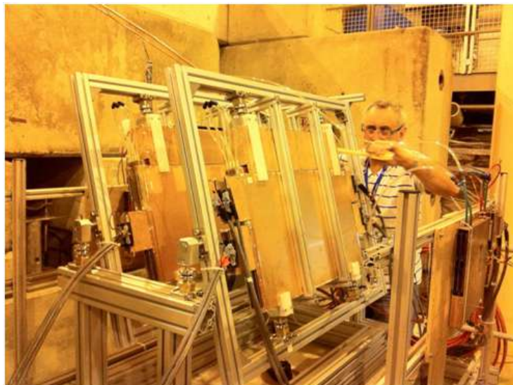
Figure 4.10: Precise mechanical set-up to align the two quadruplets and measure their characteristics for various positions and angles, with a wide beam
