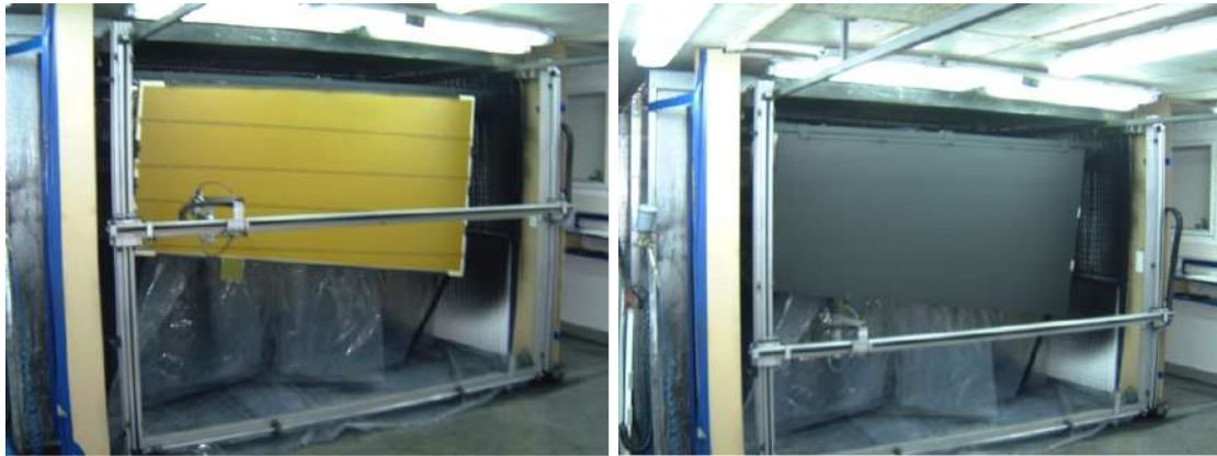
Figure 7.7: Graphite spraying. Right photograph shows graphite spray being completed for one board.
